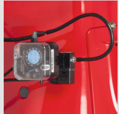
An additional solenoid valve enables the W-FM to also test the air pressure switch on burners with a continuous-run fan or post-purge facility, ensuring maximal safety
