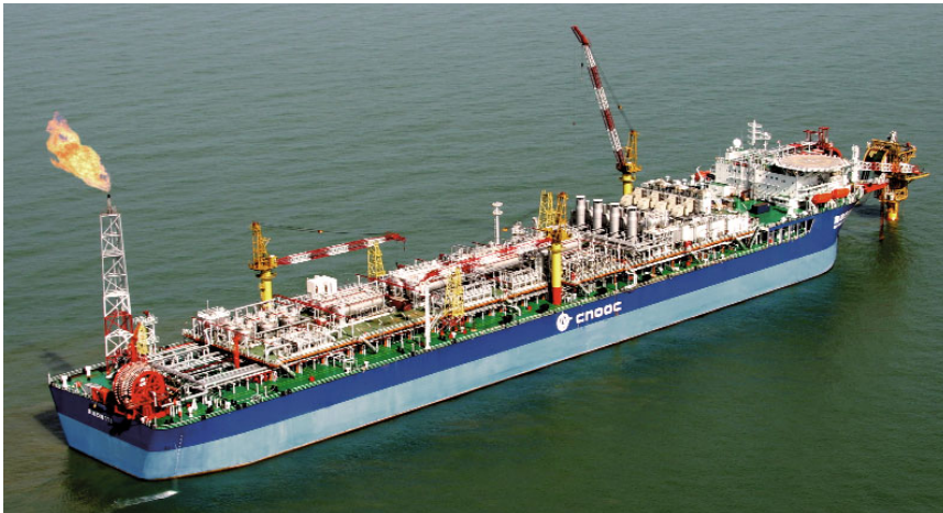
Crude oil from the drilling rigs in the South China Sea is stored temporarily on central ship depots
